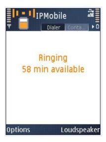
iii. While the call is ringing or after the call is connected, the user can switch to speaker mode by pressing the button below the loudspeaker as shown below
